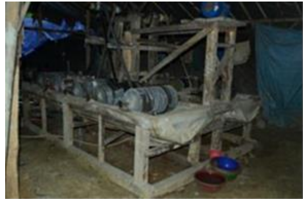
Fig. 5 Rod-mills locally called “Glondong”.
