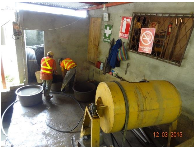
Fig. 5 Recovery gold with mercury.
